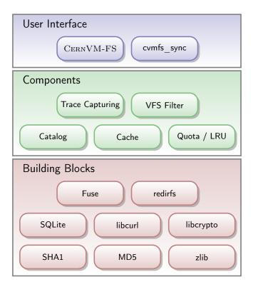
Figure 6.1.: CERNVM-FS block diagram.
