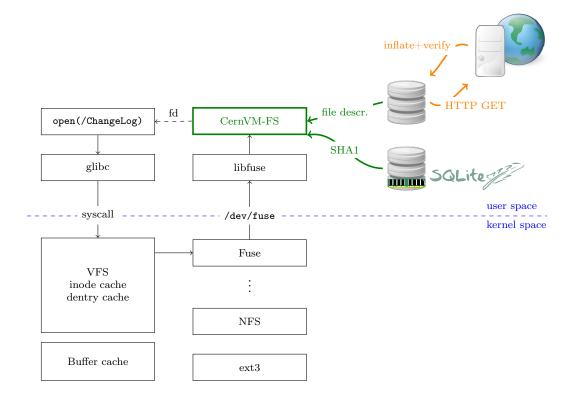
Figure 1.3.: Process of opening a file. CERNVM-FS resolves the name by means of an SQLite catalog, which is prepended by a memory cache. Downloaded files are verified against the cryptographic hash of the corresponding catalog entry. The read() and the stat() system call can be entirely served from the in-kernel file system buffers.
