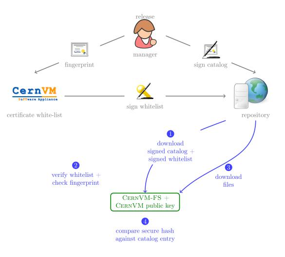
Figure 6.3.: Trust chain with a signed repository.
