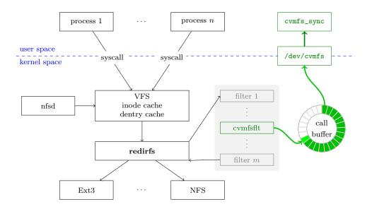
Figure 6.6.: CERNVM-FS filter for REDIRFS: Writing VFS calls are captured and written to a character device to create a file system change log.
